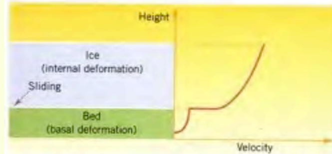
Figure 18.14 Mechanisms of glacial flow. The surface velocity of a glacier is made up from components due to internal deformation of the ice, sliding at the ice bed interface and deformation of subglacial sediments.
